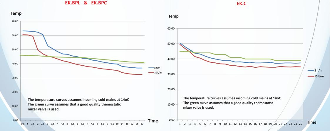
All Boilers are fully insulated ~ Instantaneous & continuous hot water ~ 230/240v single phase ~ 12kw, uses 50 Amps minimum 10 mm cable ~ Silent due to TRIAC based technology (D.E.S System) ~ can be used with radiators or underfloor heating Modulates from 2kW-12kW (Central heating) ~ Digitally displays temperatures ~ Anti-Legionella function
